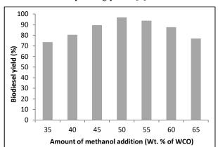
**Fig. 2.** Variation of yield with the change of methanol addition while other parameters were kept constant ( time: 90 min, Temp.: 60 °C and NaOH: 0.8 wt.%)
