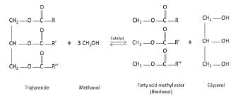
Fig. 1. A simple illustration of transesterification reaction
