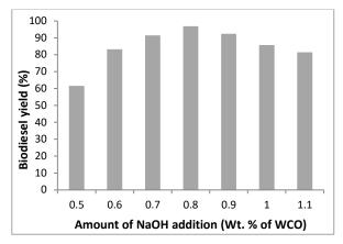
**Fig. 3.** Variation of biodiesel yield with the change of weight percentage of NaOH while other parameters were kept constant (reaction time: 90 min, Temp.: 60 °Cand methanol: 50 wt.%)
