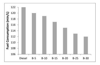
**Fig. 7:** Fuel consumption behaviour of commercial diesel and WCOB-diesel blended mixtures
