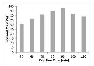
Fig. 5. Variation of WCOB yield with the change of reaction time while other parameters were kept constant (temp.: 60 °C, methanol: 50 wt.% and NaOH: 0.8 wt.%)
