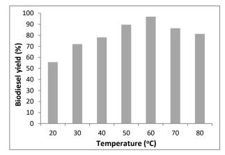
**Fig. 4.** Variation of biodiesel yield with the change of temperature while other parameters were kept constant (time: 90 min, methanol: 50 wt.% and NaOH: 0.8 wt.%)
